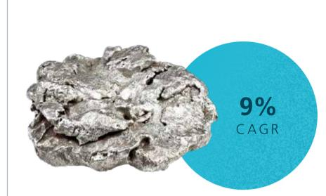
Silver is essential for contacts in solar panels as it has the highest electrical and thermal conductivity among all metals.
